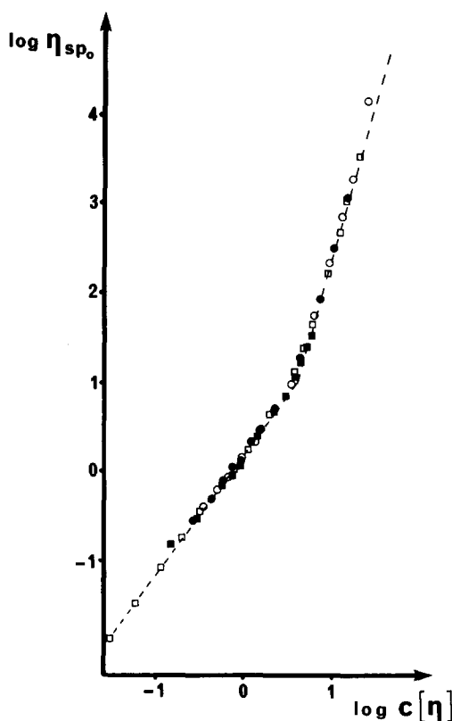
Fig. 2. Specific viscosity at zero shear rate ( \eta_{sp0} ) as a function of c[\eta] : ■, CMC 7LXF; □, CMC 9M65; (●) sodium alginate and (○) \lambda -carrageenan from Goncalves (1984); ---, Morris et al. (1981) for dextran, carboxymethylamylose, alginates, \lambda -carrageenan and hyaluronate (pH 7.0, 0.015 M NaCl).
